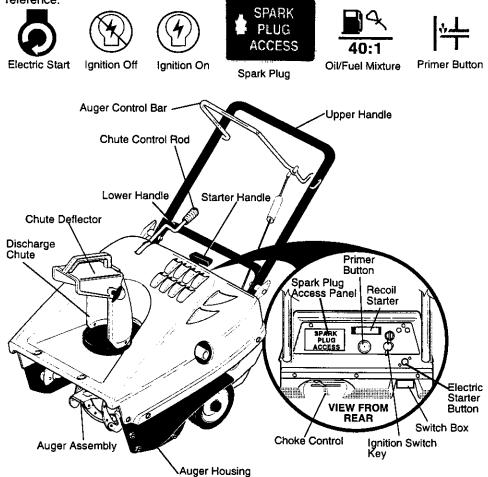
Auger Control Bar – Starts and stops the auger which propels the snow thrower. Chute Control Rod – Changes the direction of snow discharge.
